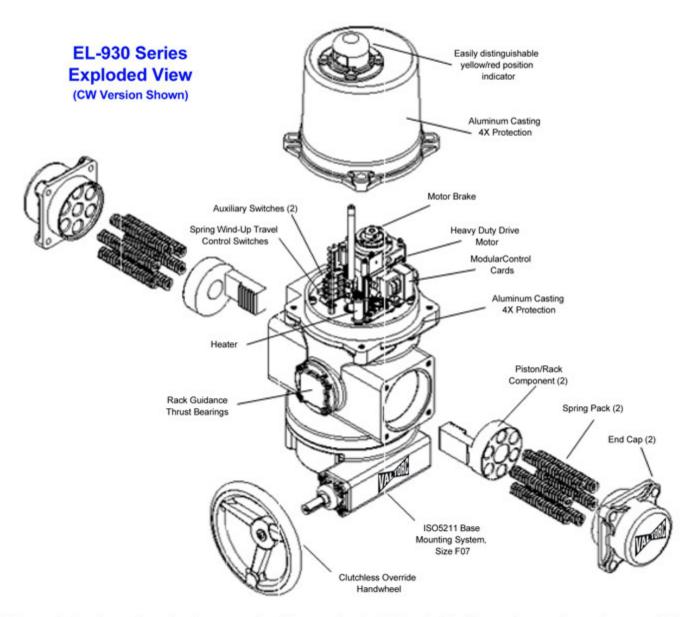
A modular cast aluminum housing incorporates the mechanical drive train, the spring pack, rack assemblies, output drive shaft, motor and control section and the manual override handwheel unit. The spring pack is NOT field servicable and spring failure direction mode must be selected at time of order.
