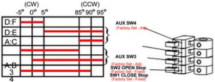
Switch/Cam arrangement for Jog & Proportional control (CW Version shown)
