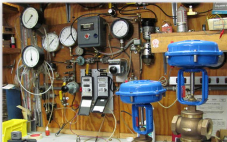
THE PICTURE TO THE TOP RIGHT SHOWS THE PRESSURE CALIBRATION STATION. MECHANICAL AND DIGITAL ELECTRONIC TEST INSTRUMENTS HAVE AN ACCURACY OF 0.1% FSD AND ARE TRACEABLE TO NIST STANDARDS IN CALIBRATION AND ACCURACY.
