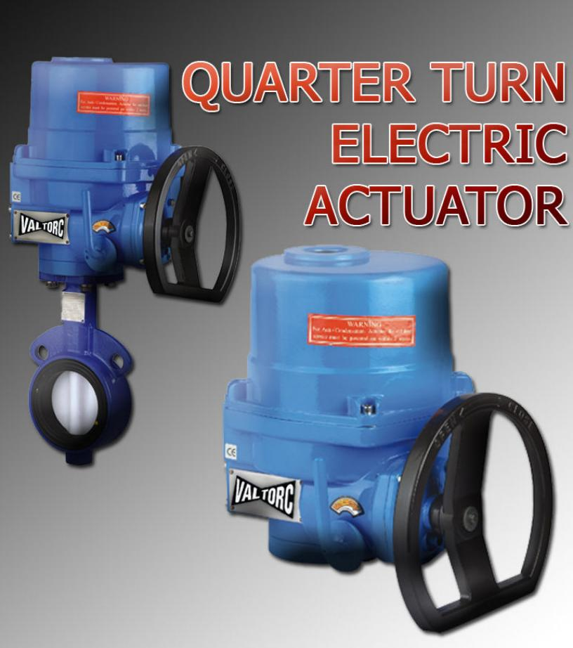
The VALTORC Electric Actuator is designed and engineered for robust, reliable and high performance duty on quarter turn valves. The unique reliable motor module, adjustable cam plate limit switch, self locking mechanism, precision gearing system and ball bearing, auto declutchable mechanism, light rim pull on the hand-wheel, adaptor drive bushing and bottom ISO 5211 mounting dimension are added advantages against others in the field of valve automation. CE approved. FM & UL pending.
