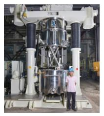
apply intense shear to achieve a smooth, uniform consistency. The PDDM is rated for vacuum operation up to 29.5 in. Hg and includes a jacketed changecan vessel, sight/charge ports on the cover and an automated lift for raising and lowering the agitators. **Charles Ross & Son Company**
